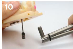
10 Remove the Pliers from the Insertion Pin.
