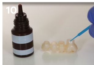
10 If applicable, apply the ceramic primer to the restoration. The ceramic primer can be used for Zirconia (ZrO 2 ) glass ceramics, porcelain, composite, Ti and CoCr.
