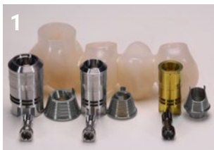
1 Overview of components for the manufacture of the cement jig.
