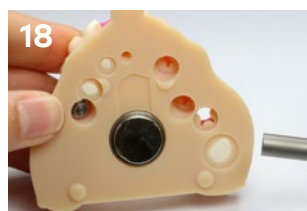
18 Remove the Pliers and the installation procedure is done. The Analog is now perfectly seated in the 3D printed model.
