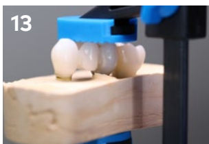
13 Place the bridge structure on the Universal Bases Non-Engaging covered with cement and mounted on the jig.
