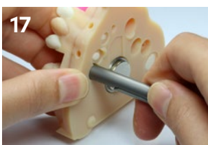
17 Rotate the Pliers clockwise until the Insertion Screw is fully screwed. The torque applied to the Insertion Screw must not exceed 5 Ncm. (Screw lightly.)
