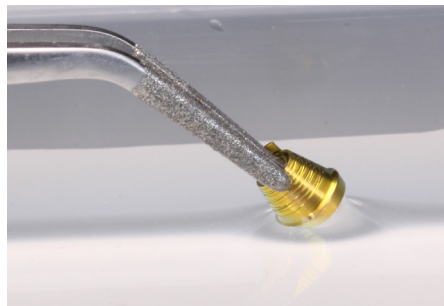
2. Before cementing, clean the surface thoroughly with alcohol 99.5% (<95% alcohol) or KATANA™ Cleaner.
